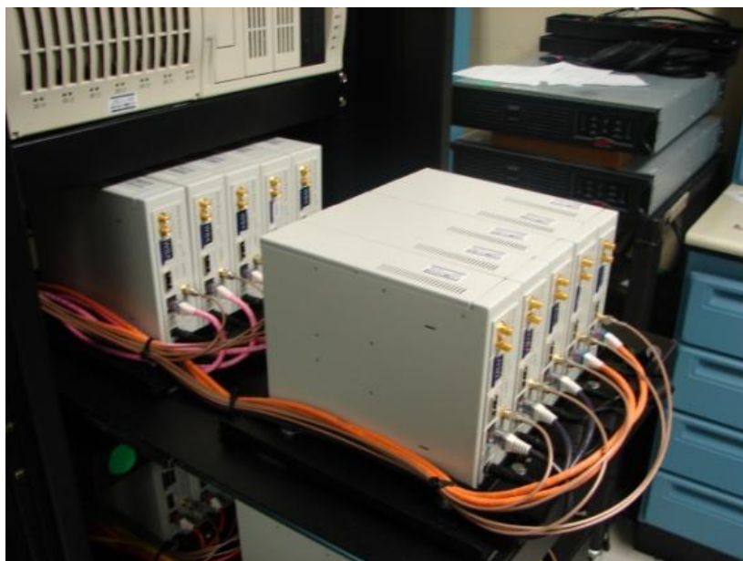
USRP2s Installed in the 64 Node Testbed
